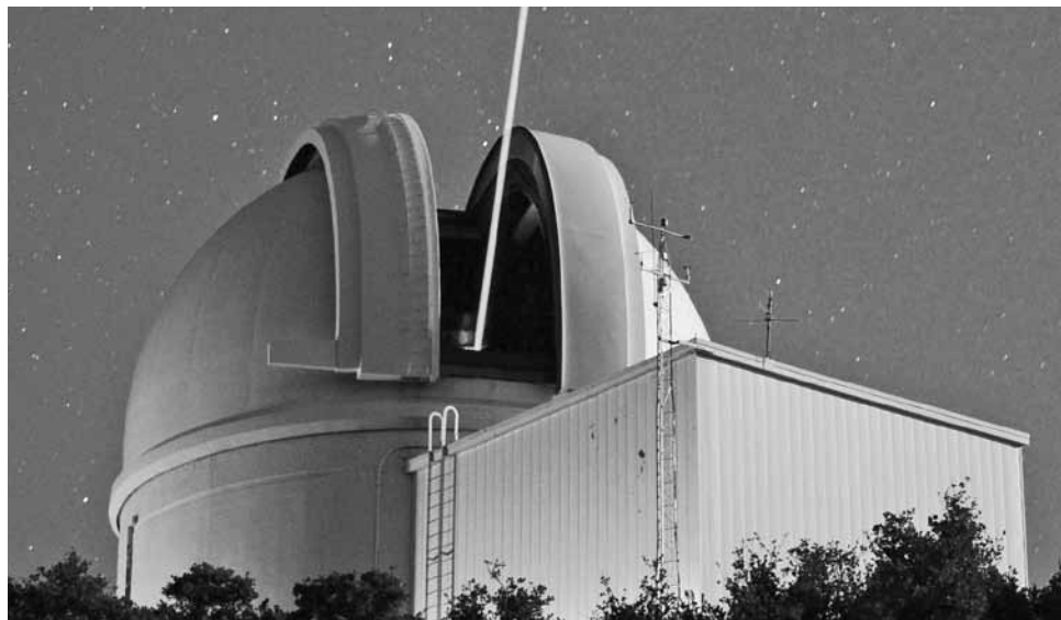
"The ultraviolet Robo-AO laser originating from the Palomar 1.5-meter Telescope dome. (Although the laser is invisible to the human eye, it shows up in digital SLR cameras once their internal UV blocking filters are removed. The apparent color of the laser beam is a result of the UV light leaking through the camera's red, green and blue pixel filters by slightly different amounts.)" – University of Hawaii Institute for Astronomy. Photo Credit: C. Baranec.
