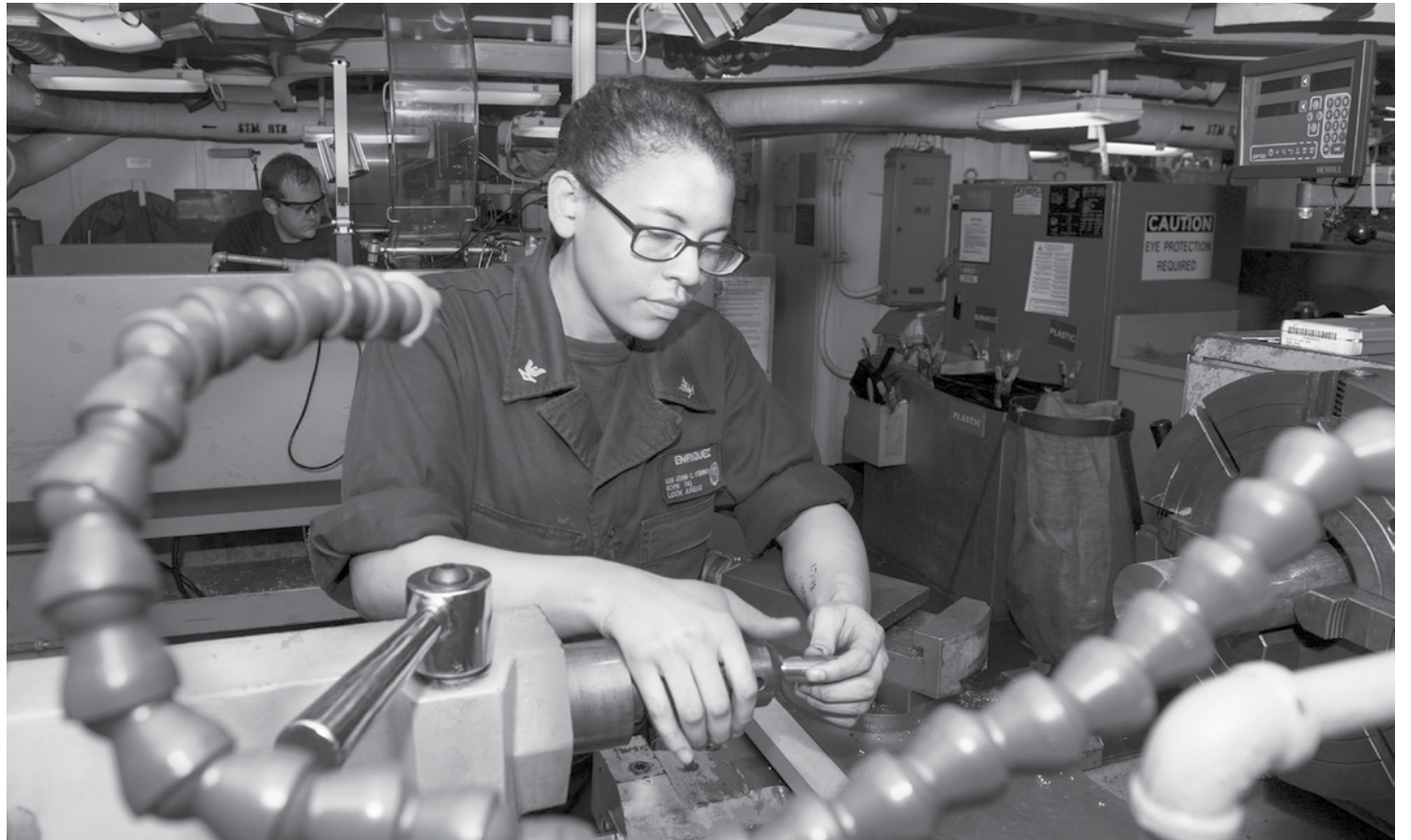
Machinery Repairman 3rd Class Hamali Enriquez from Los Angeles, re-threads a valve stem in USS John C. Stennis' (CVN 74) repair shop. Providing a ready force supporting security and stability in the Indo-Asia-Pacific, John C. Stennis is operating as part of the Great Green Fleet on a regularly scheduled 7th Fleet deployment. U.S. Navy photo by Mass Communication Specialist 2nd Class DeAndrae McDaniel
